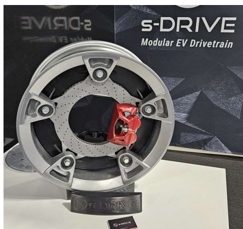
14. ábra s-DRIVE in wheel motor [55]
