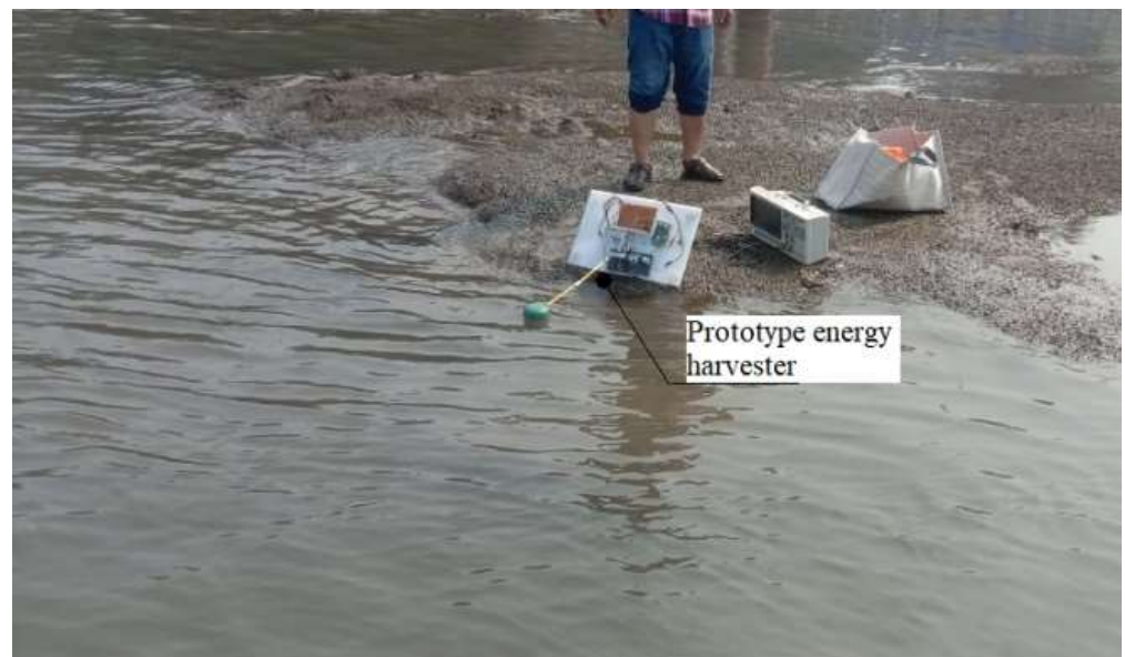
Figure 15. Experimental arrangement for energy harvesting along the seacoast.
