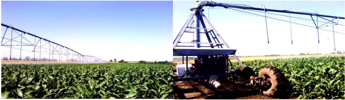
Figure 18. Linear sprinkler irrigation system at Látókep Research Station (Debrecen, 2018)
