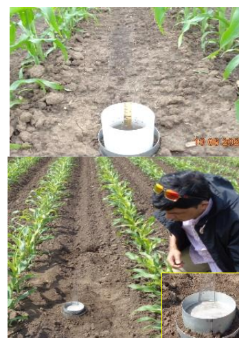
Figure 20b. Infiltrimeter (Debrecen, 2020)
