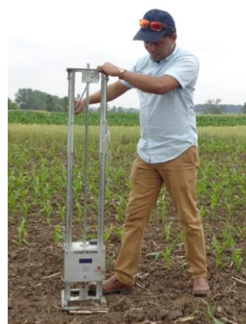
Figure 20a. Penetrometer (Debrecen, 2020)
