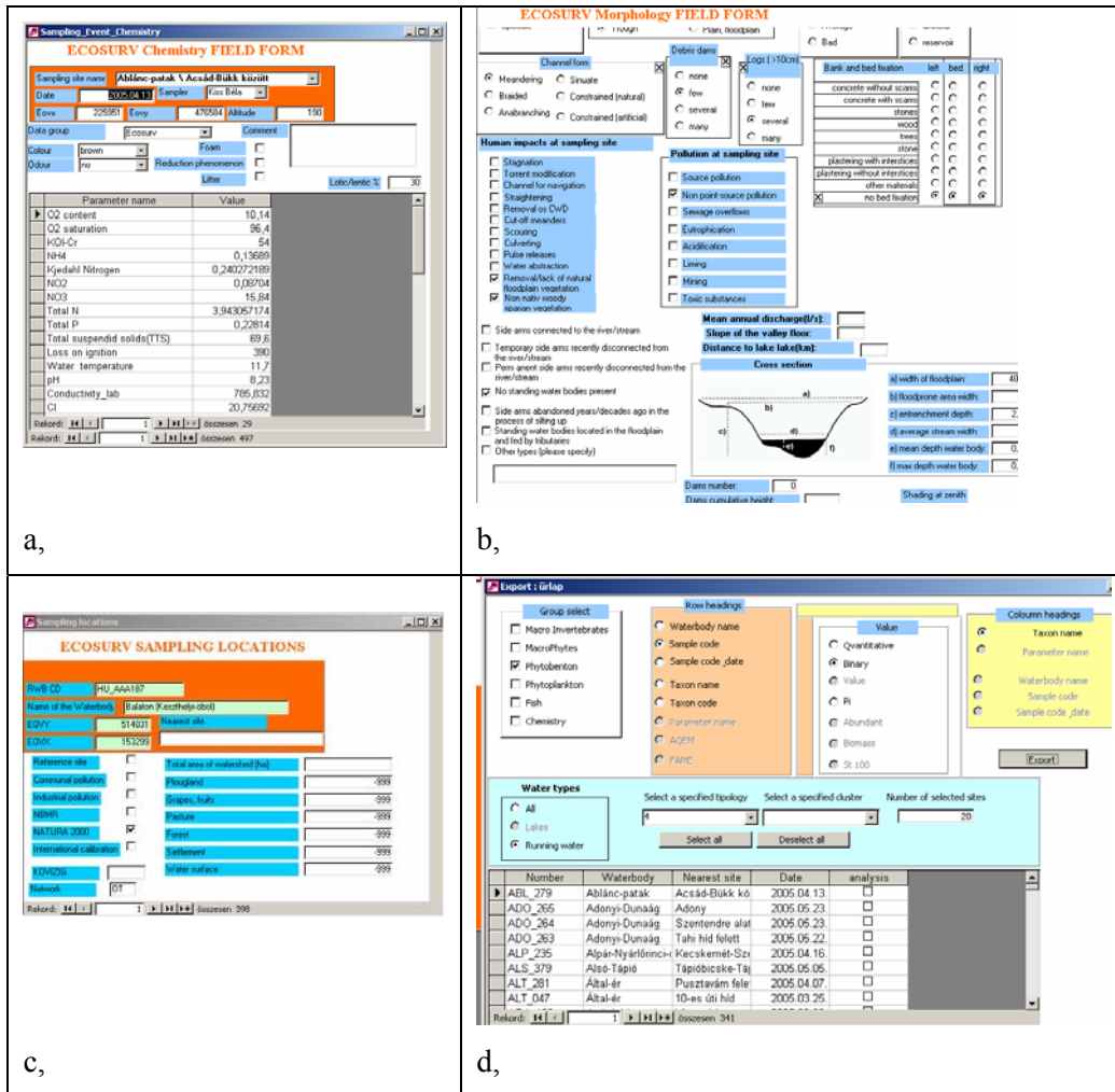
Fig. 7. Selected forms from the ECOSURV database, a, Chemical sampling events form; b, hydromorphological information; c, Sampling locations form; d, Data export form.
