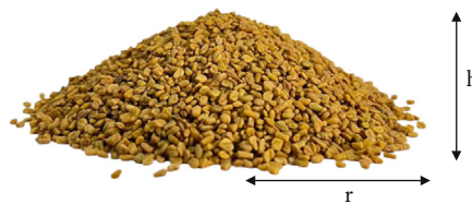
FIGURE 1: Pile of fenugreek seeds for determination of angle of repose. The lines labeled “h” and “r” represent the geometric dimensions of the cone-shaped seed pile. Specifically, “h” denotes the vertical height of the pile, while “r” indicates the base radius, which are used for calculating the value of angle of repose, i.e., \theta .
