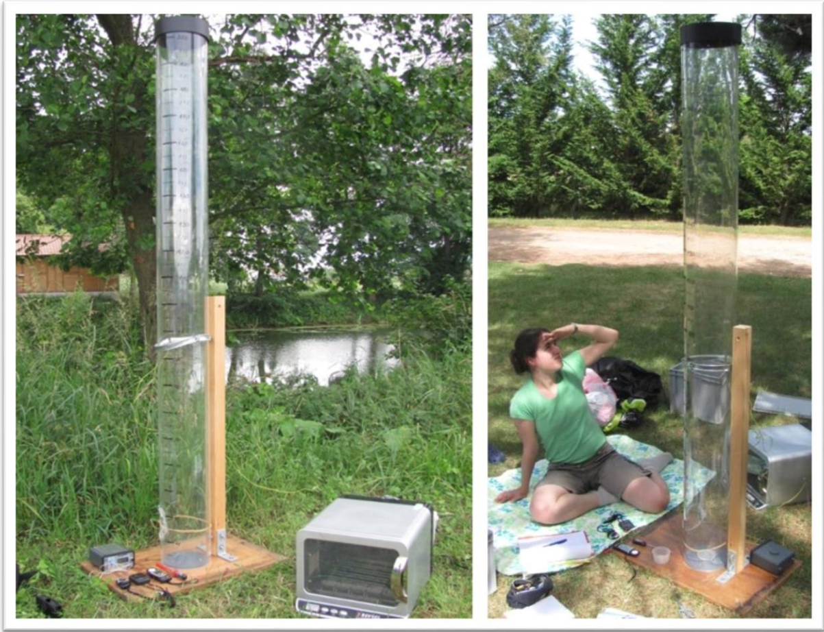
Figure 5. Experimental set-up to quantify flight performance of damselflies in the field. The transparent Plexiglas flight tube (height: 2 m, diameter: 20 cm) was placed vertically, connected with a metal ring to a wooden mainstay and was fixed on a wooden ground plate for stabilisation. The top of the tube was covered with a grey non-transparent lid. The cup containing the animal was placed at the bottom of the tube and the lid of the cup was gently removed at the start of the flight test. (Photo credit: Lieven Therry)
