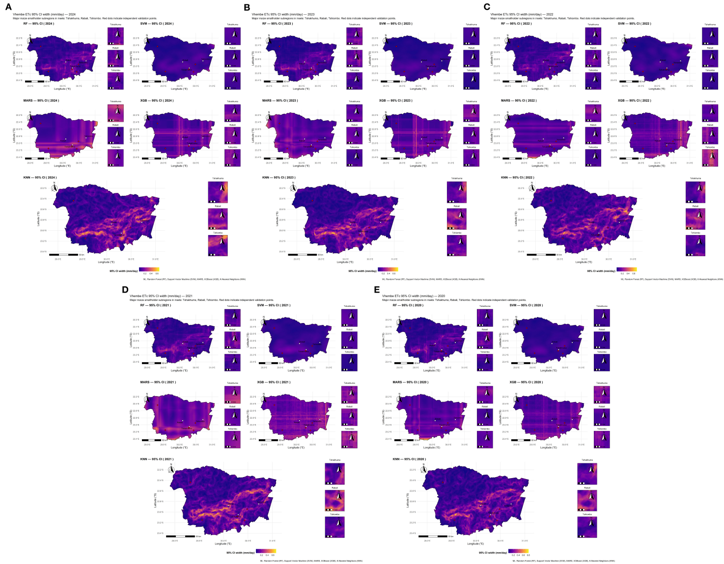
FIGURE 8 Spatial prediction of daily maize evapotranspiration (ET c , mm/day) across Vhembe District for (A) 2020, (B) 2021, (C) 2022, (D) 2023, and (E) 2024, with performance comparison of five machine learning models: K-nearest neighbors (KNN), random forest (RF), support vector machine (SVM), multivariate adaptive regression splines (MARS), and extreme gradient boosting (XGB).
