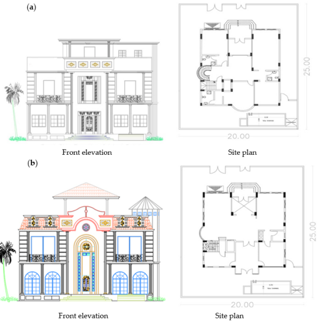
Fig 3. (a) Original design front elevation (left) and the typical site plan (right). (b) Modified design front elevation (left) and the typical site plan (right).
