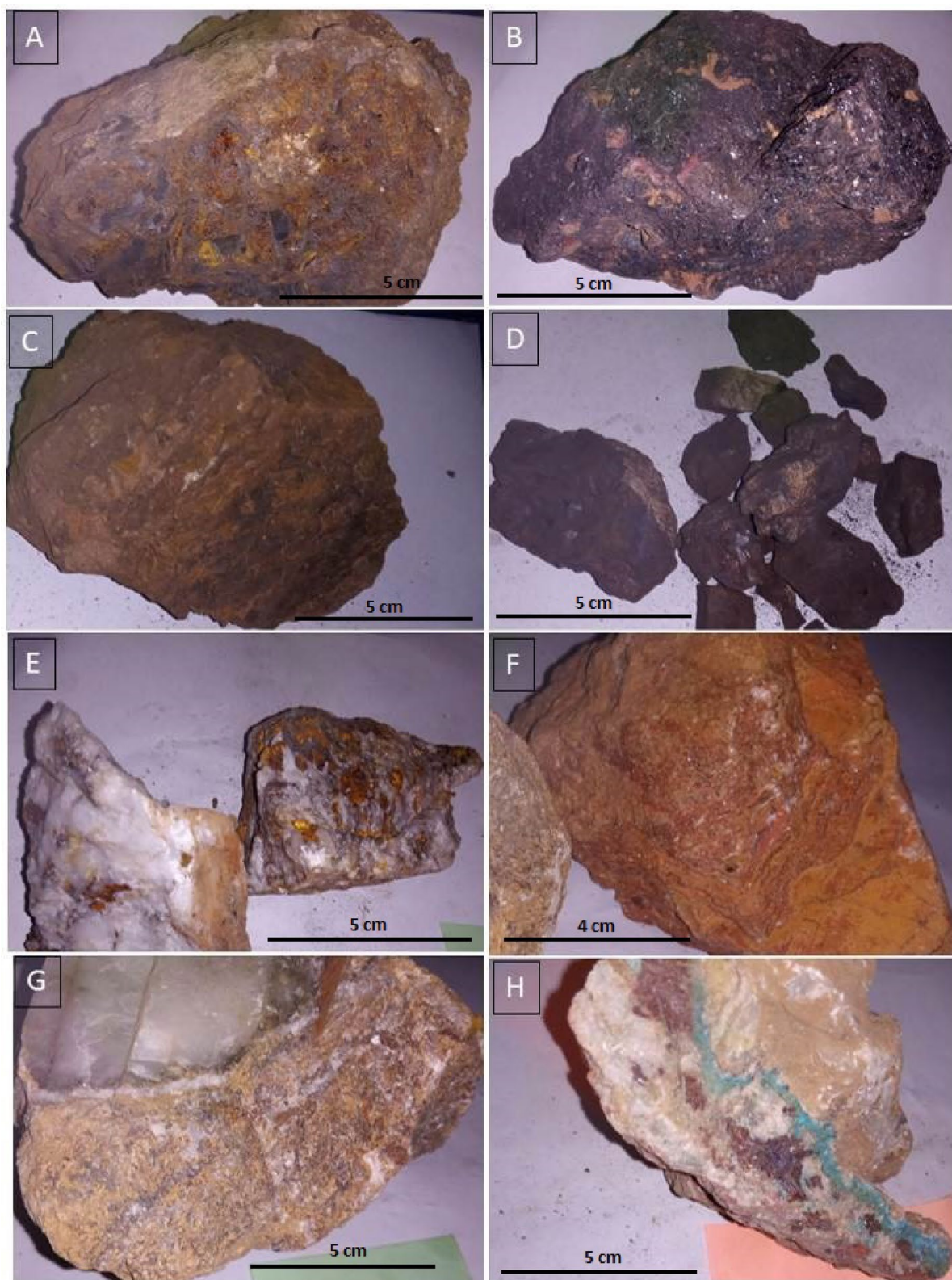
Fig. 10. (A)–(C) smithsonite associated with P21 iron oxides. (B) sphalerite P29. (D) Manganese ore P28. (E) Quartz with iron oxide inclusions. (F) Smithsonite with P21 iron oxidation. (G) Zn smithsonite ore with P21 calcite crystals. (H) Origin of malachite associated with iron oxides P26. P refers to the field station point.
