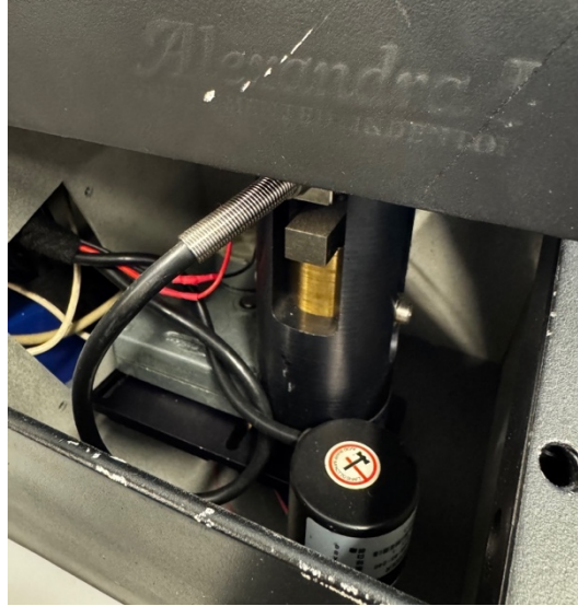
Figure 52 Motor-actuator system that controls the machine
