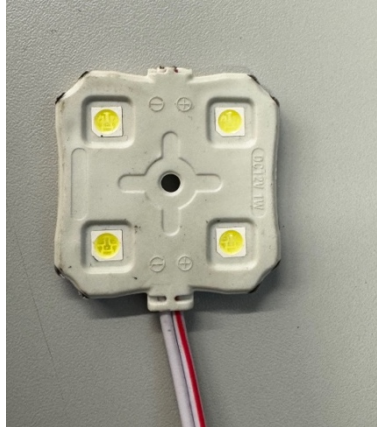
Figure 58 LED light used for our DIC equipment
