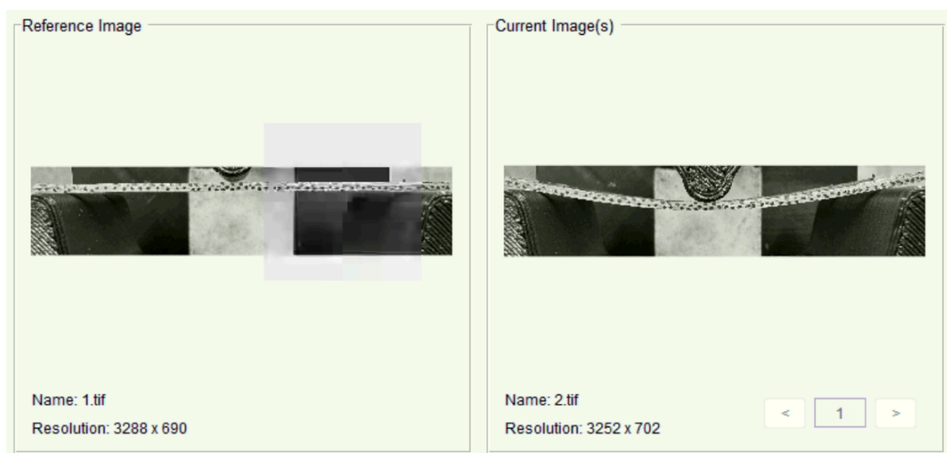
Figure 73 Reference image and deformed image uploaded to Ncorr
