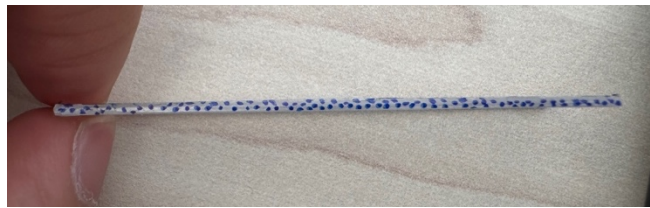
Figure 67 Speckle pattern applied to the surface of the specimens
