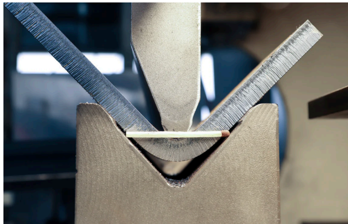
Figure 24 Bending test in a ductile material (Source: [7])
