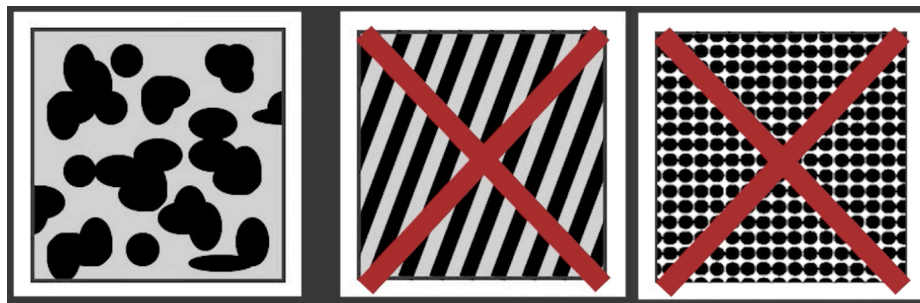
Figure 38 Correct form of speckle patterns on the specimen surface (Source: [37])
