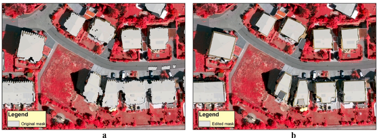
Fig. 2. Result of the building masking (a: original mask; b: edited mask; background image: orthophoto of Vaihingen).
