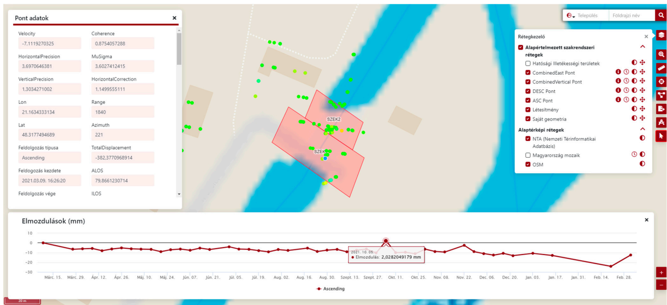
Figure 11. Interactive user interface, with the objects of a water facility and their PSs. The time series and quality measures of the chosen PS are highlighted on the left side and bottom of the figure. The layer handling toolbox is on the right side of the figure. The displayed PS points are mostly stable (green color), while some shows a slight displacement towards the sensor (yellow color). Please note, that this interface is in Hungarian, so the decimal separators are commas, not periods.
