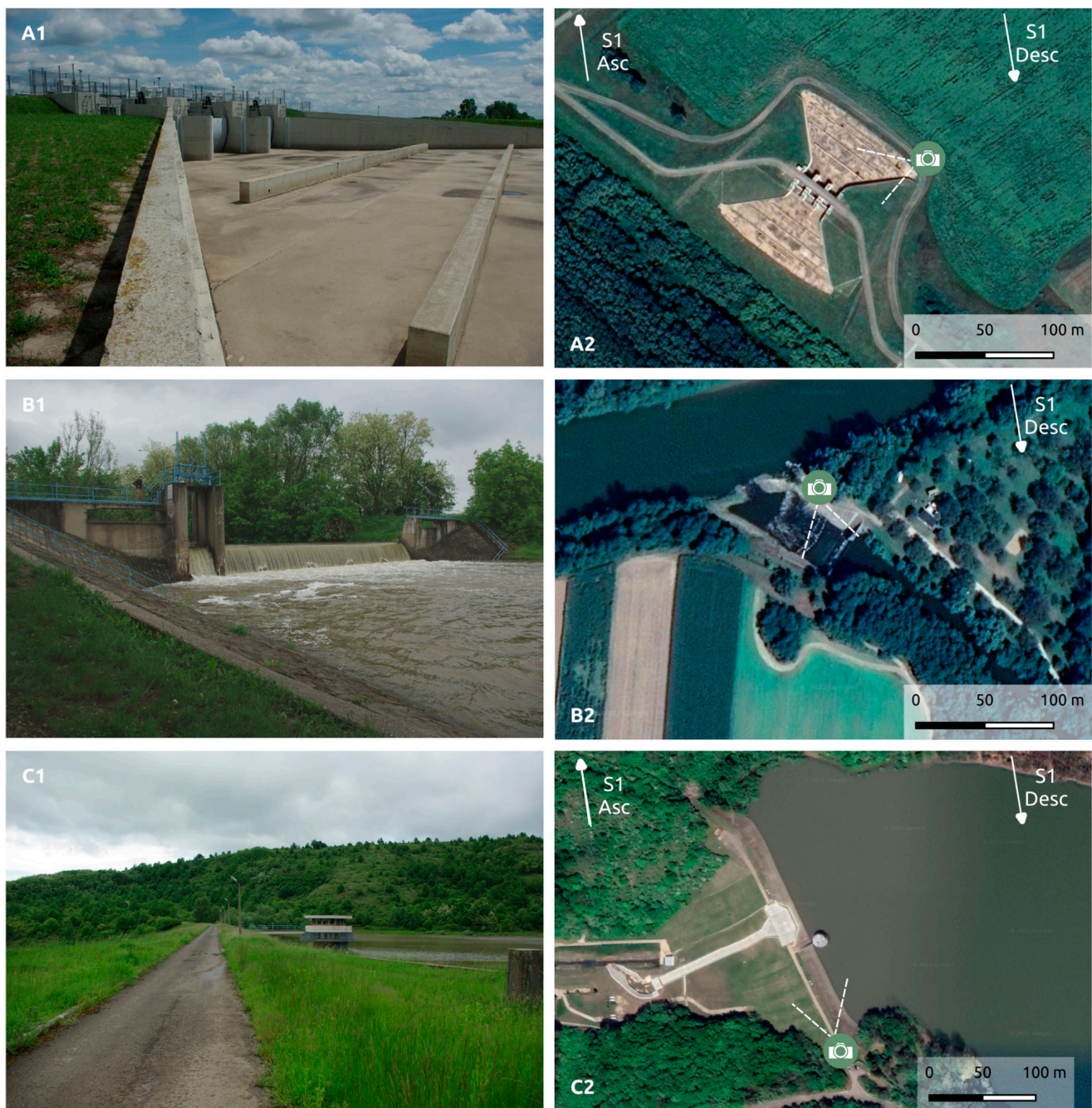
Figure 5. Typical detectable (A1), undetectable (B1) and improvable (C1) sites and their land cover from Google satellite images (A2–C2). Typical PS densities of site types are the following: undetectable site = 0 PS (but improvement is impossible with CR), detectable = usually 5 + PS, improvable = from 0 to 5 (but improvement is possible with CR).
