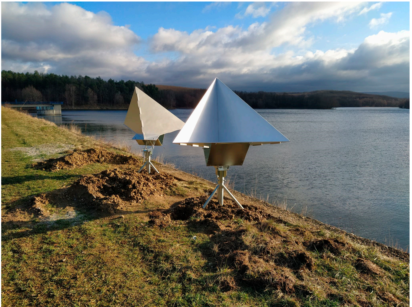
Figure 6. CR pair facing both ascending and descending S1 orbits on a reservoir dam (the overflow drain is in the upper left corner of the picture). Check Figure 7 for localisation.
