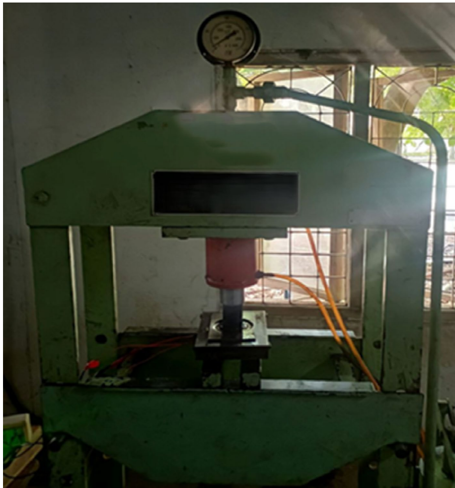
Fig. 4 Compression molding set up with a hydraulic press
