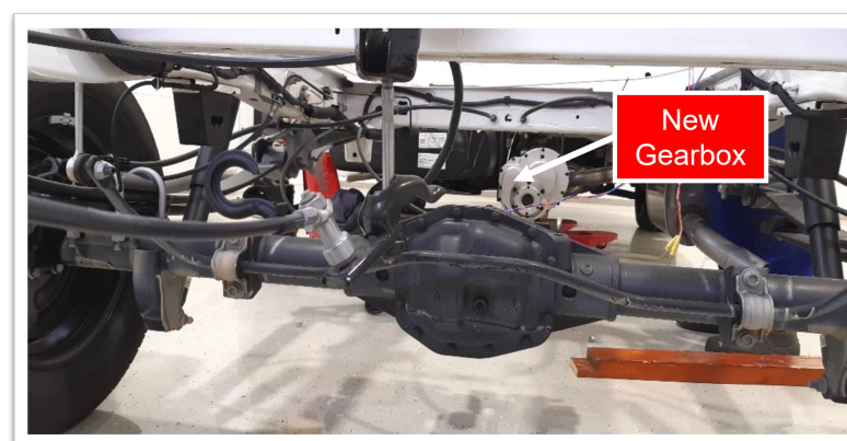
Figure 10. New Gearbox Location on the Vehicle adapted from [45].
