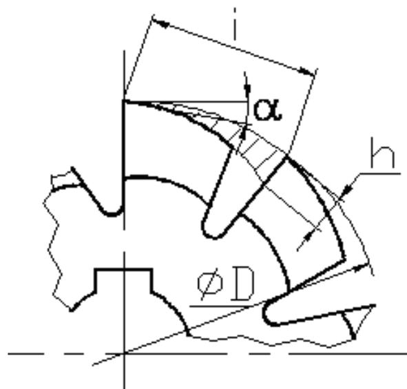
Figure 7. Defining of dimension of the backward turning
