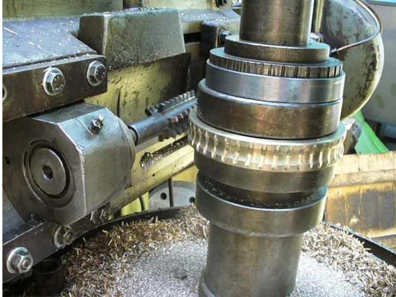
Figure 2. Worm gear production
