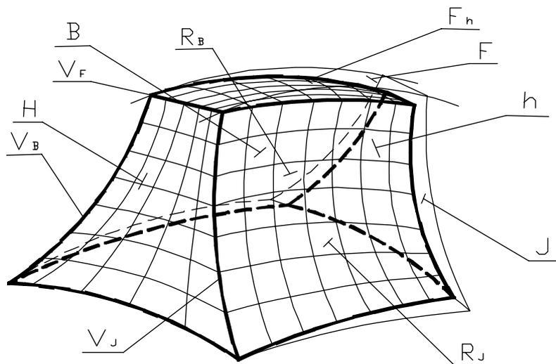
Figure 3. Surface elements and edges of hob
