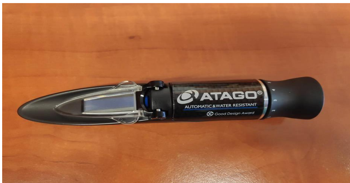
Figure 21. Refractometer (Source: From Laboratory, Institute of Food Science, University of Debrecen, Manufacturer- Atago )
