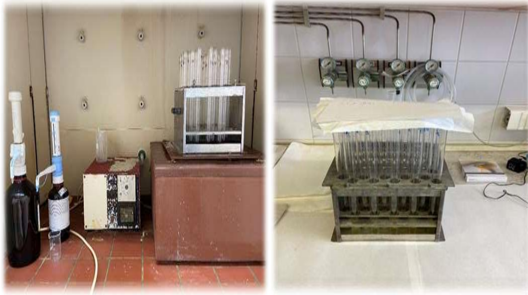
Figure 23. Digestion unit and tubes (Left Fig A. Digestion unit with Nitric acid and Hydrogen peroxide, Right Fig B. Digestion tubes with samples for green walnut and other samples). (Source: Picture from Laboratory, Institute of Food Science, University of Debrecen).
