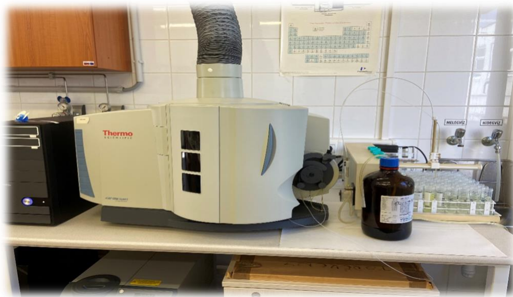
Figure 24. Inductively Coupled Plasma Optical Emission Spectrometer (ICP-OES) (Source: Picture from Laboratory, Institute of Food Science, University of Debrecen).
