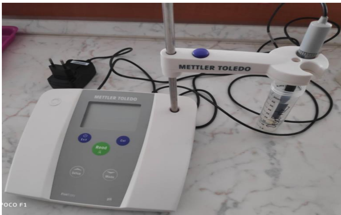
Figure 22. Digital pH meter (Source: From Laboratory, Institute of Food Science, University of Debrecen, Manufacturer- METTLER TOLEDO)
