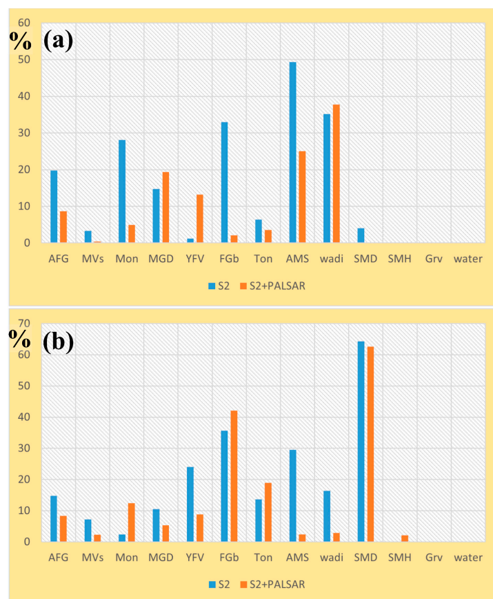
Figure 7. Errors of commission utilizing (a) Sentinel 2 and (b) the combined PALSAR Sentinel 2 datasets.
