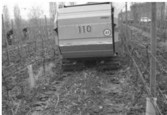
Figure 1: Vineyard pruning harvesting by a round-baler
