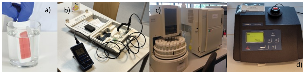
Figure 2. a) HygieneCheck PLUS test; b) Multiline P4 meter (temperature, conductivity, salinity, T.D.S.) c) Shimadzu TOC-Vcph device (T.O.C.), d) Turb 555IR light scattering photometer (Turbidity)
