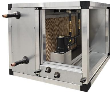
Figure 4. Prototype of an evaporative cooling device integrated with the source-side heat exchanger of a liquid-coupled air-handling unit
