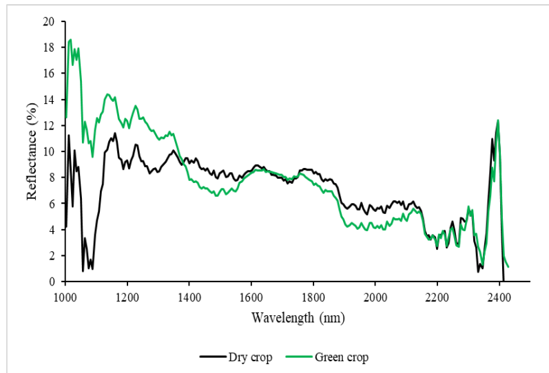
Fig. 6. Evolution of reflectance of dry and green crops in the wavelength range 1000-2500 nm
