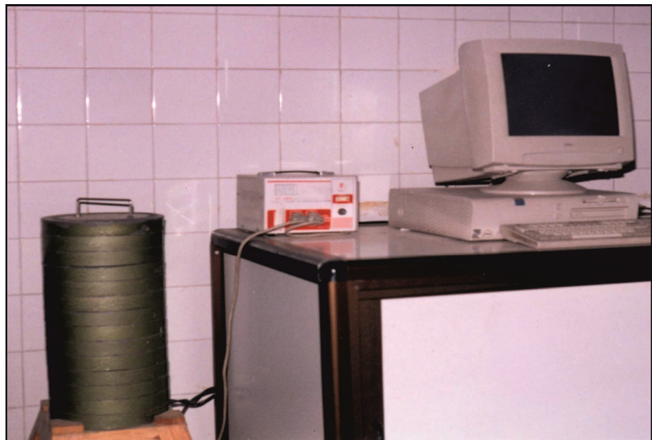
Figure 5. Na-I detector. Source: Research Division. Geochem. Exp. Dept. NaI Laboratory, Nuclear Materials Authority (NMA), Egypt.
