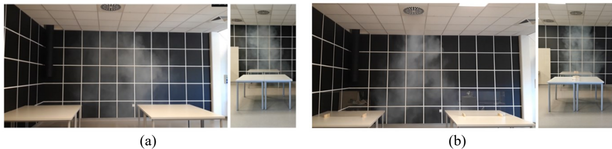
Figure 4. Airflow pattern at the workstation setup with 4 desks, (a) with empty desktops, (b) with plexiglass sheets on the desktops
