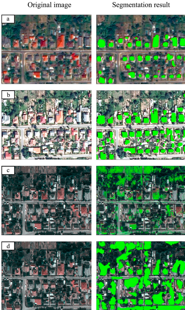
Figure 4. Segmentation results when the training dataset and the predicted image were the same. – a) 2-P40-2; b) 0-P40-0; c) 3-P5-3; d) 3-P10-3. First and last tags of the labels: 2 = WorldView-2; 3 = WorldView-3; 0 = Orthophoto. Second tag = Number of training image used for the prediction (before augmentation).
