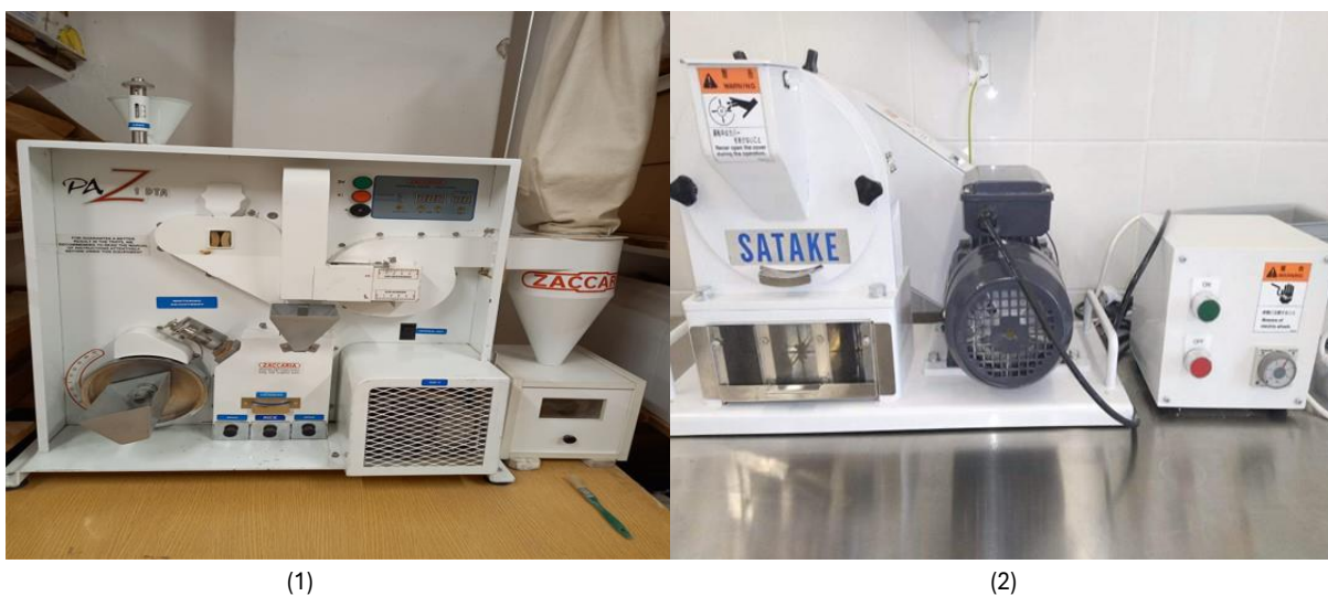
Figure 2. The utilized huskers (1) Zaccaria No. 1. testing rice mill for 60 (S), Institute of Research, Karcag. (2) Satake husker for the husking technique, Lab of Food Science and Technology
