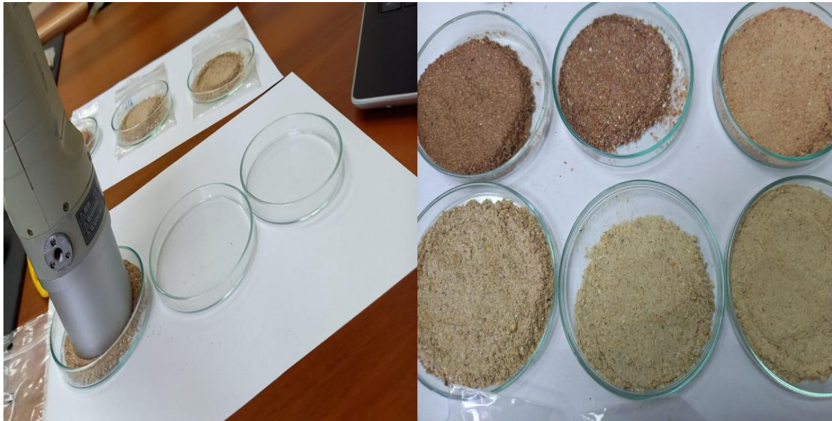
Figure 3. Measurement of the colour profile of the respective grain varieties by utilization of CR-410 Konica Minolta Camera
