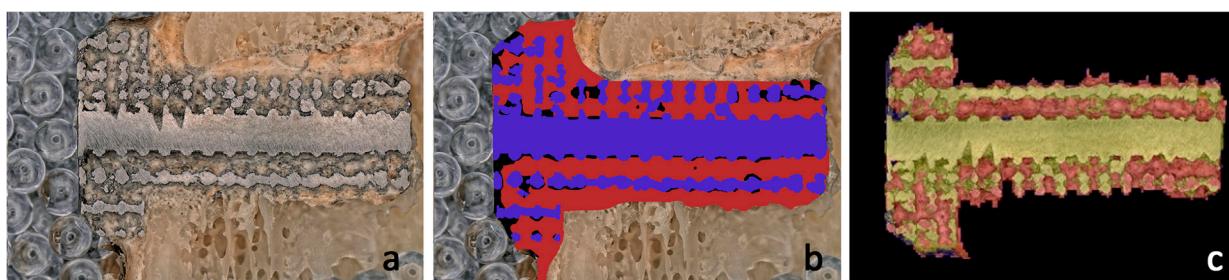
Figure 10. Analysis of bone ingrowth shown on an optical microscopic image of a cube grid test specimen: (a) image shows the original input picture; (b) image shows the result obtained by manual drawing; (c) image shows the result obtained by the image processing algorithm.
