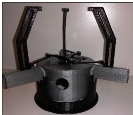
Fig. 4. The finished gripping tool on the holder
