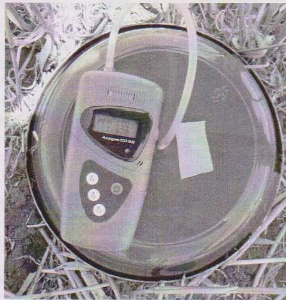
Figure 1. The ANAGAS 98 infrared gas analyser
