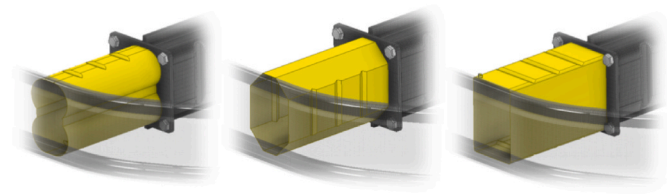
Fig. 19. The notched versions of the crashbox specimens (Authors).
