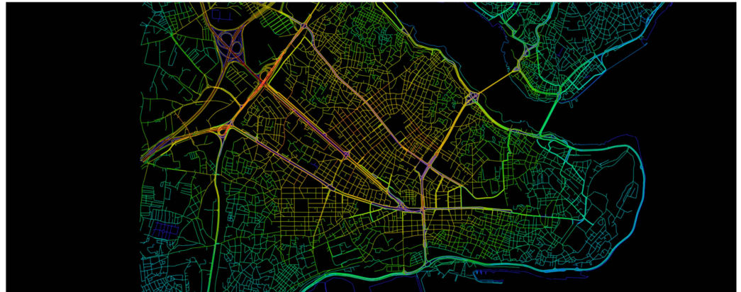
Figure 8. Configuration features of route structures. The degree of configuration for each segment line is depicted using a gradually sifting color scale. The red axes represent the highest configuration and dark blue donates the lowest configuration levels. The map is generated from the Space Syntax Toolkit plugin in QGIS 3.4.4.
