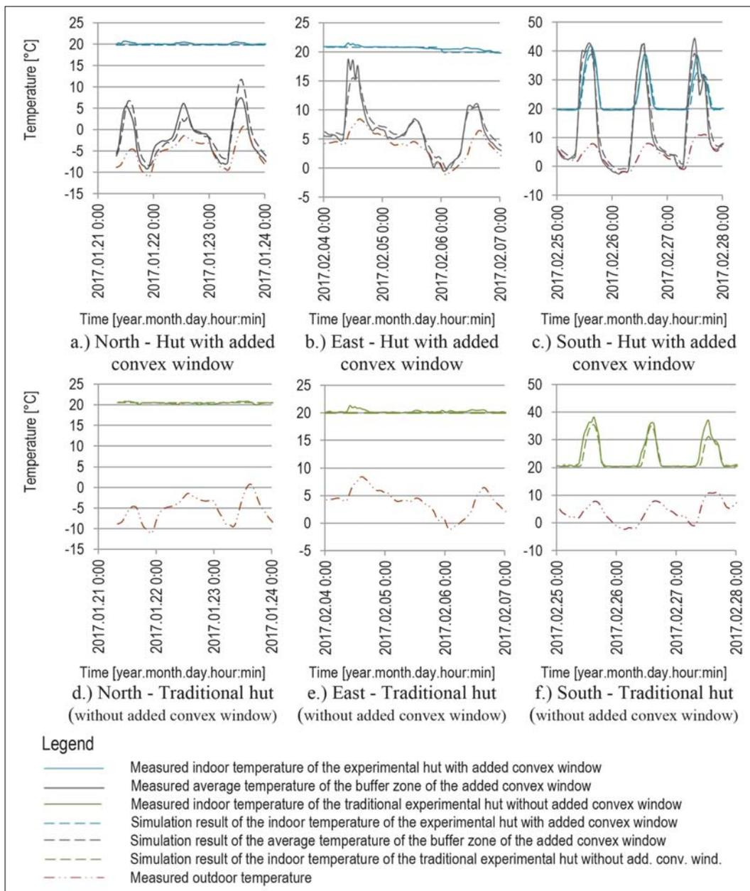
**Fig. 6.** Results of temperatures from simulations and measured data (Time: Central European Time, CET)
