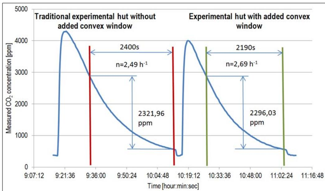
Fig. 5. Measured data of the CO<sub>2</sub> concentrations and the air change numbers
