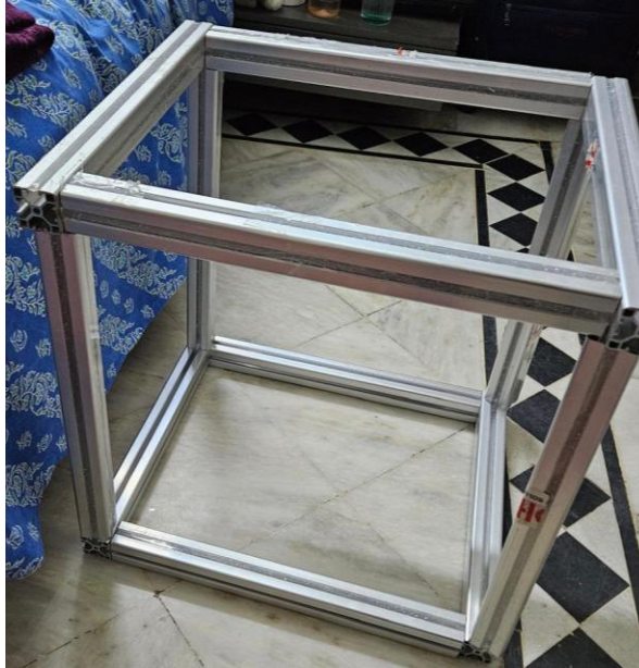
Fig.29 shows the 40x40 aluminum extrusions.
