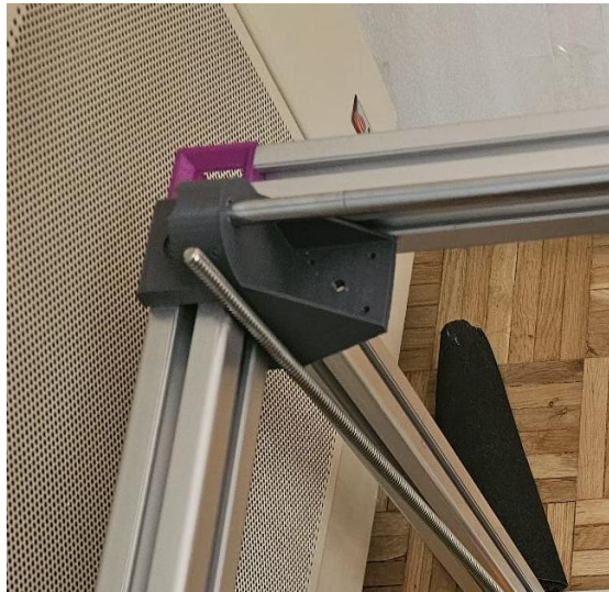
Fig. 49 shows the motor mount fitted into the frame.
