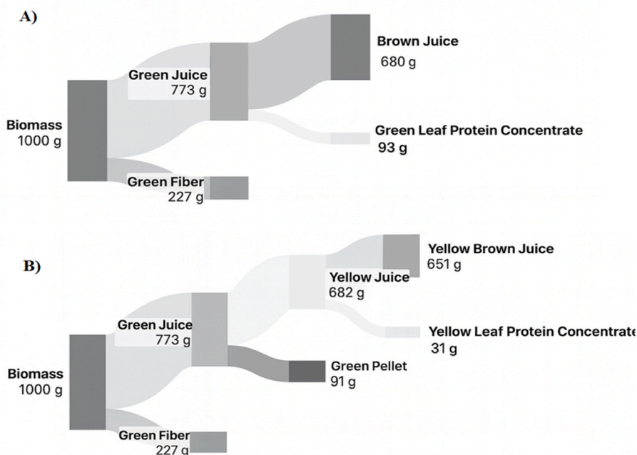
Fig. 2. A) Yield of wet fractionation to obtain fresh green leaf protein concentrate (MW-GLPC) and by-products B) Yield of wet fractionation to obtain fresh yellow leaf protein concentrate (YLPC) and by-products. Data are presented as mean \pm SD (n = 3).
