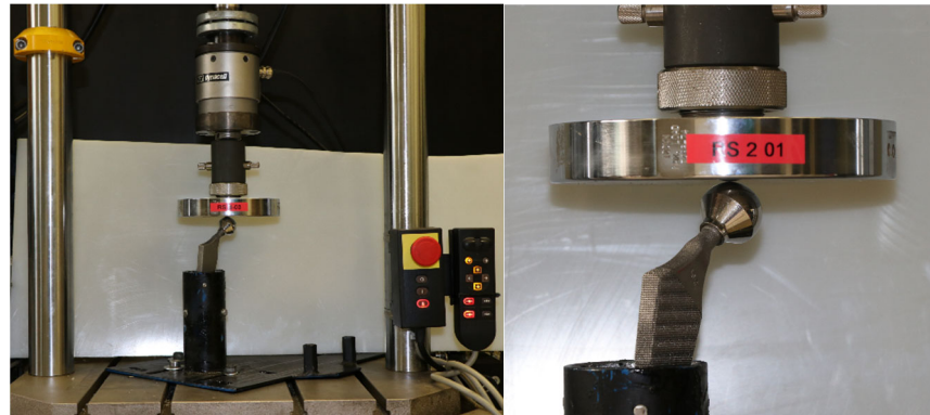
Figure 9. Hip implant compression test setup.
