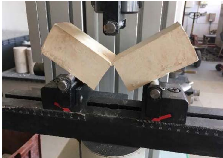
Fig. 5. Damage of sample No. 0 1 after the flexural strength
