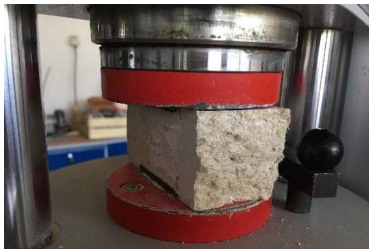
Fig. 6. The sample No. 7.5 12 during the compression strength test
