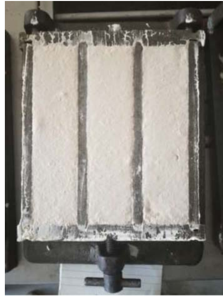
Fig. 4. Mixture of test specimens in test mould
