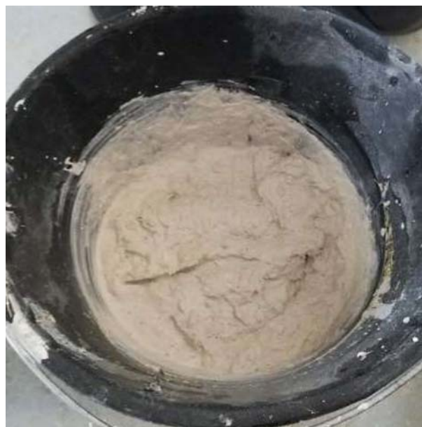
Fig. 2. Mixture of plaster with wooden fibers
