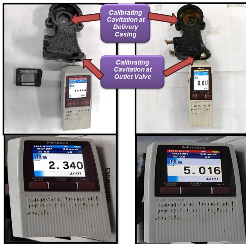
Figure 4. Calibrating: Good condition impeller casing and cavitated impeller casing.
