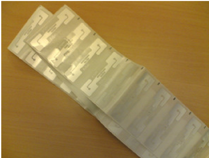
Figure 1. About a hundred EPC Class 1 Generation 2 sticker tags, just as they left the factory.
