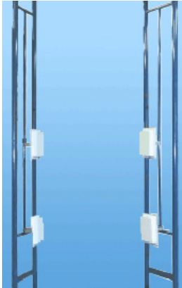
Figure 8. The layout of a regular UHF gate, with two antennas on both sides.
