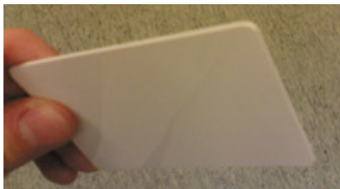
Figure 2. An ISO 15693 HF tag that is indistinguishable from a regular plastic card.
