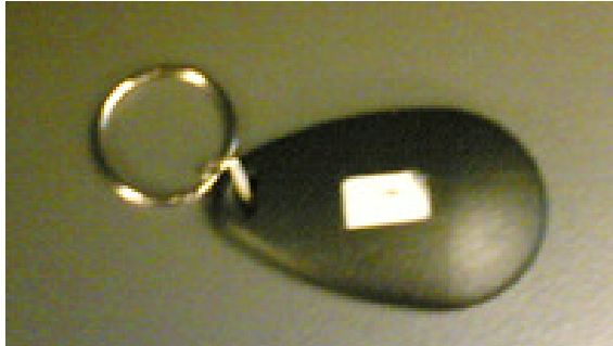
Figure 3. A tag for low-frequency RFID.
