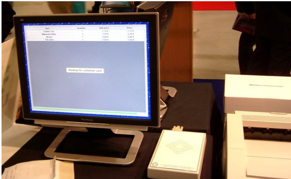
Figure 18. The display with the presentation application, the HF reader used to detect customer cards, and the printer used to print receipts.
