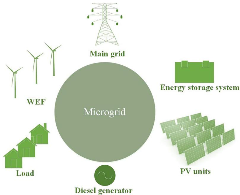
Fig. 1. The structure of a sample MG
