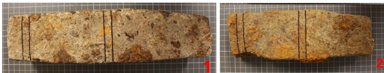
Fig. 1: Marking of sampling locations for iron bars 1 and 2. Two slices were made from each sample for a complete examination of the objects.
