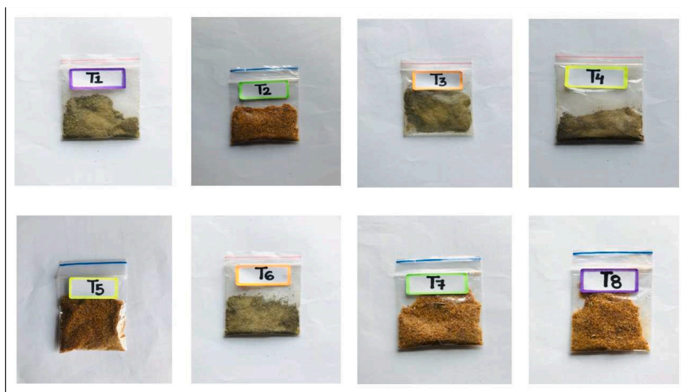
Fig. 4. Chitosan powder extracted from mushroom waste powder using microwave assisted extraction technique.
