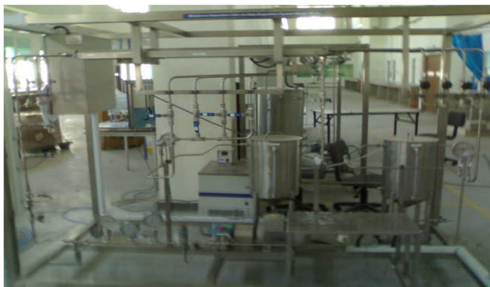
FIGURE 6 | Membrane separation unit TR-14.
