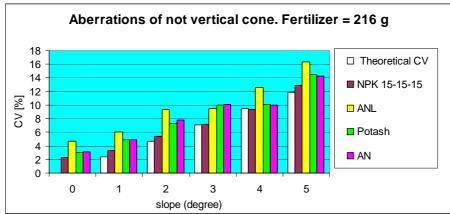
Figure 4: Result of examination the cone-belt dispenser
