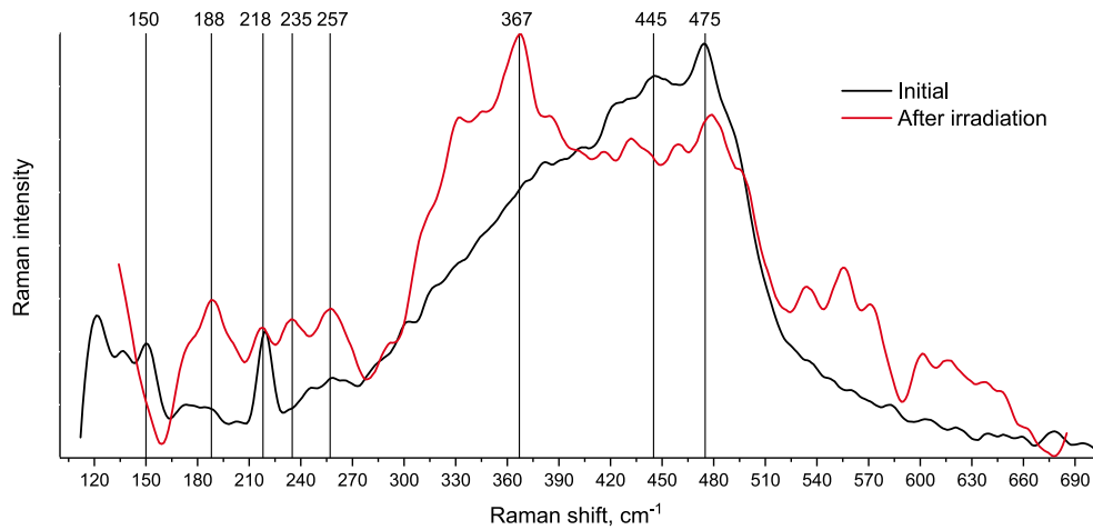
Fig. 2. Raman spectra of PG-As 2 S 3 before (black curve) and after irradiation with 532 nm laser (red curve). (For interpretation of the references to colour in this figure legend, the reader is referred to the web version of this article.)
