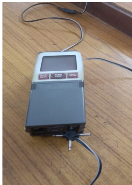
Fig. 3. Surface roughness tester.
