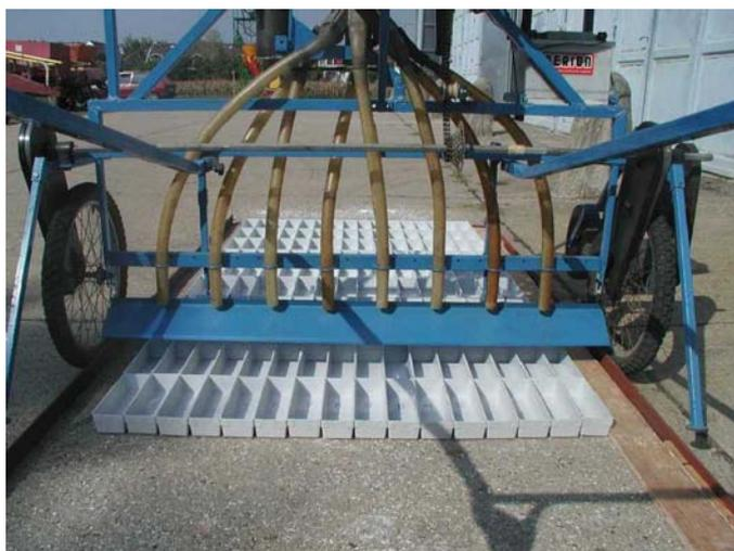
**Picture 4. Examination of unevenness of spreading with testing trays placed on whole surface**
