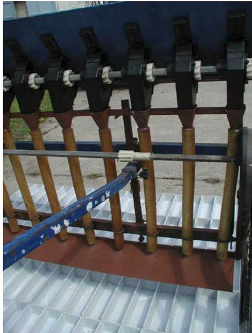
**Picture 1. getting the fertilizer near the ground by the converted FIONA/1.5 Plot Fertilizer**
