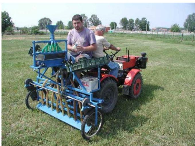
**Picture 9. The designed and developed experimental plot fertilizer distributor**
