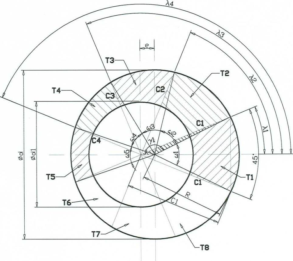
**Picture 6. The territories of the segments (T1...T8) between the feeding cylinder (d) and the cone dispenser (d<sub>1</sub>)**
