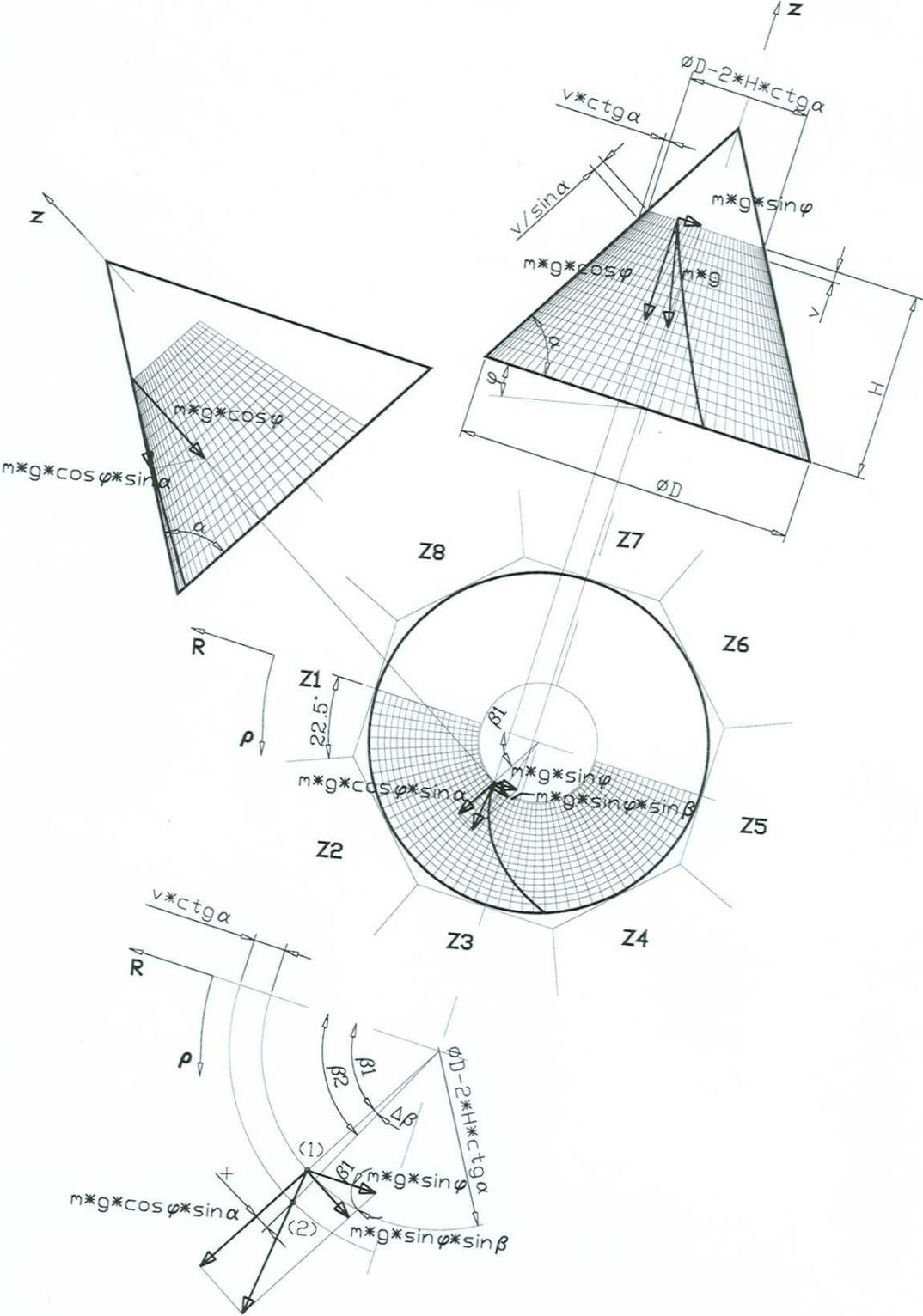
**Picture 7. The movements of fertilizer on the not horizontal cone**
