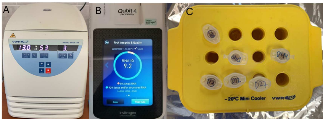
Figure 12. Sample preparation and RNA integrity check: A: Centrifuge, B: Invitrogen Qubit 4 Fluorometer, and C: mini cooler box.
