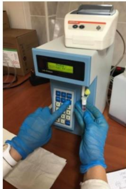
Picture 2. Measurement of samples using the Lab-Analyse spectrophotometer
