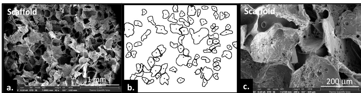
Figure 8. (a) SEM images of SO-PU3 scaffold; (b) the outlines of the pores examined; and (c) zoomed SEM image of SO-PU3.
