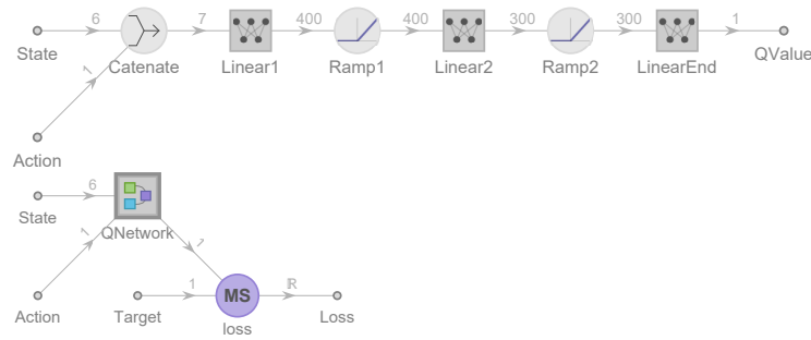
Figure 17. The architectures of Q-network and training network to update the Q network.
