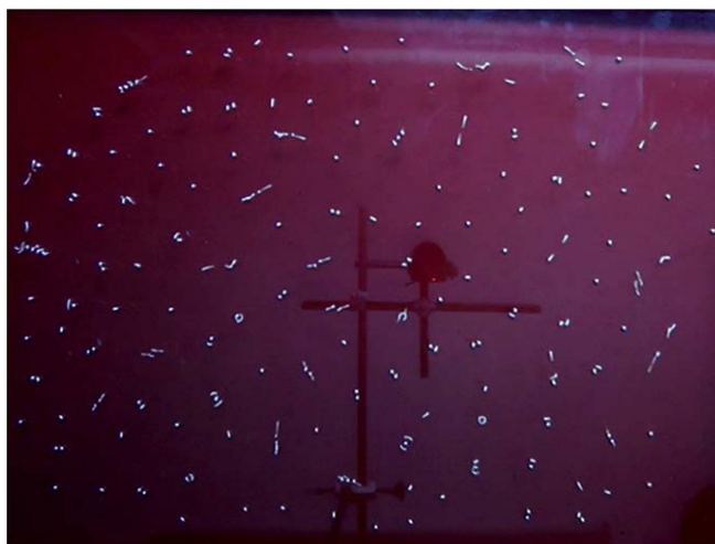
Figure 2. 0.08 s after the drop/start. There are still solitary, motionless balls. Several cases of pair-interactions and formation of pairs – dimers – are observable. In some cases, non-linear movement of the balls can be noticed. The central collisions are creating slow-moving dimers, while non-central collisions are resulting in quickly rotating dimers. Formation of three ball chains – linear trimers – are also observable by the interaction of dimers and single balls. Some of the trimers are also rotating.
