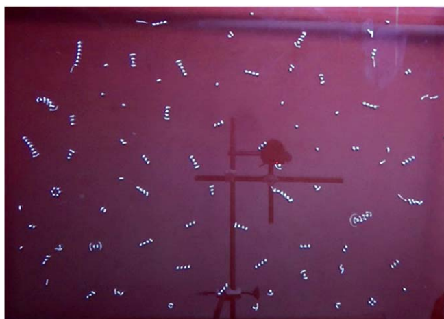
Figure 4. 0, 18 s after the drop: longer chains of 4–8 balls are forming. Some of the chains are strongly vibrating, wobbling, the blurred picture of some balls suggest large kinetic energy. On the left side in the middle, a 6 ball ring, on the lower right side a 4 ball ring was formed of short chains.
